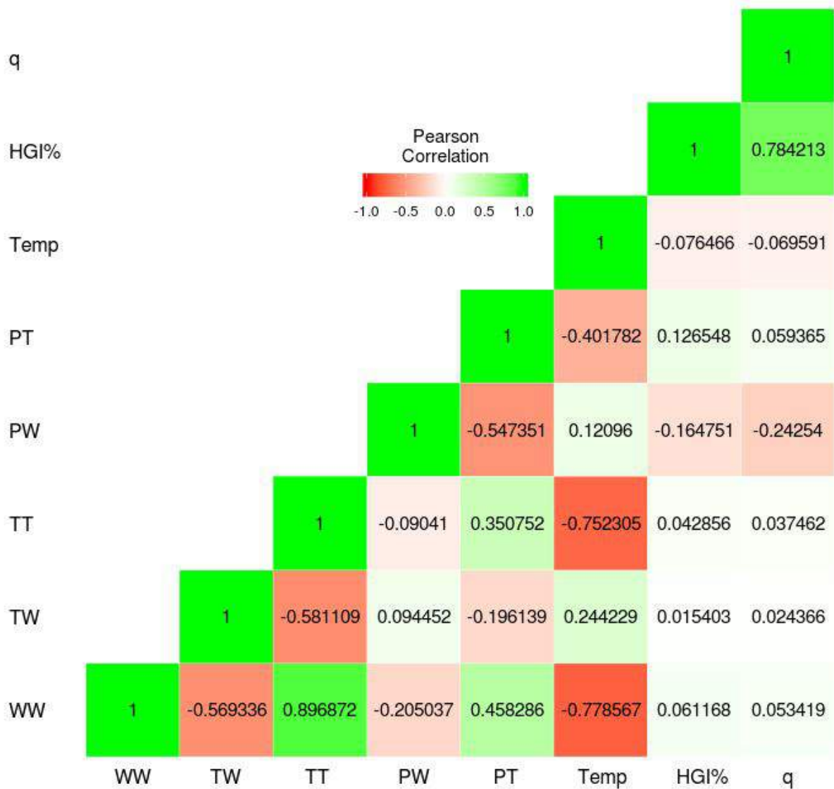
Figure.8.1 Presentation of the correlation among contact pairs of the simulation in a data heatmap matrix calculated based on Pearson's correlation coefficient factor r including only the temperatures [280K-320K] of file. The matrix and calculations were made with R program using the libraries reshape2 and ggplot2 45 . This figure is another version of Figure.8.1 in pg. 24 . In this version the correlation matrix was not reorder using the function hclust .
