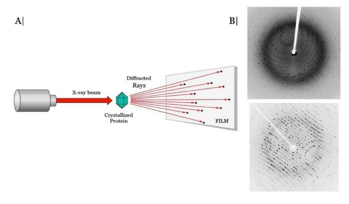
**Figure 22** | **A.** *The X-ray Crystallographic Experiment* **B.** *Diffraction patterns (above & below); The black dots indicate the reflections of the crystal.*
