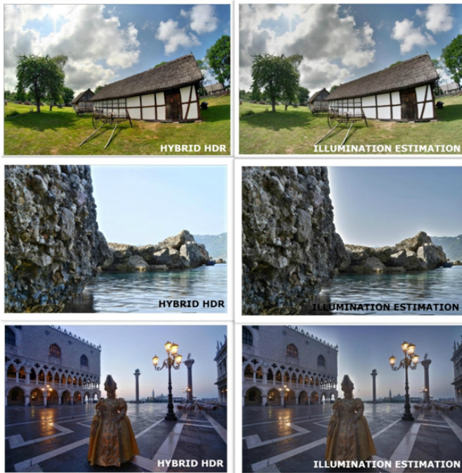
Fig. 4. Comparison between the HybridHDR and the Illumination Estimation method for three image sets. One can see more halo artifacts in the Illumination Estimation method.
