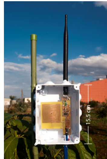
Fig. 3. An experimental prototype of the proposed self-powered wireless sensor, constructed using off-the-shelf electronic components.
