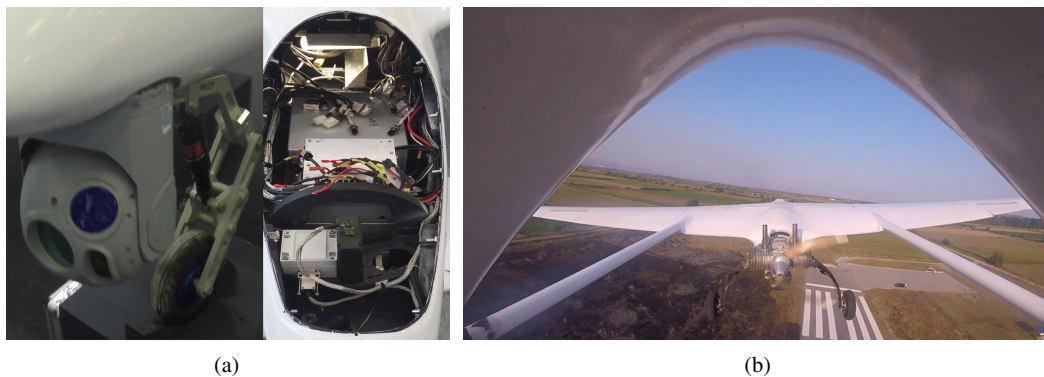
Figure 2. The HCUAV electro-optical airborne sensor system. a) Infrared and day camera gimbal with its electronics compartment; b) Actual test flight.
