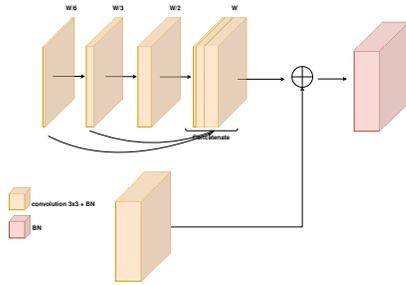
Fig. 3. The MultiRes block used in the U-Net concept.
