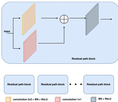
Fig. 4. The Residual path used in the MultiRes Visual Attention U-Net.
