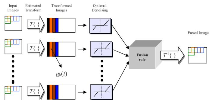
**Figure 1.** Proposed image-fusion framework.  $T\{\}$  and  $T^{-1}\{\}$ : Independent-component analysis (ICA)-trained transformations and their inverse.  $\underline{u}_k(t)$ : Image coefficients in the ICA domain.
