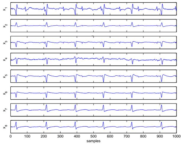
Fig. 3. ECG signals taken by abdominal ( $x_1 - x_5$ ) and thoracic ( $x_6 - x_8$ ) measurements from a pregnant woman [1], [3].
