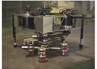
Fig.12: Hull cleaning robot, Hiroshima Univ. *www.naoe.hiroshima-u.ac.jp/staffs/hirata/img*
