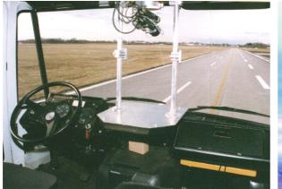
Fig.1: Unmanned car developed by Ernst Dickmanns at UniBW München; field tests with speeds up to 180 km/h, automatic passing of cars, automatic avoidance of potholes, automatic turning into cross-roads
