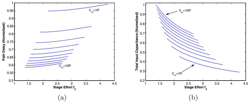
**Fig. 3.** (a) The delay and (b) the total input capacitance of an example path for various values of stage effort  $f_2$ . The path consists of three inverters in the first chain and one in the second. The wire and the loading capacitance are 50 and 100fF, respectively
