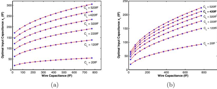
**Fig. 2.** Optimal and estimated input capacitances of the second chain for various final loads and wire capacitances. The path input capacitance is assumed to be 5fF. (a) The case with three inverters in the first chain and one in the second. (b) The corresponding case with three inverters before and after the wire
