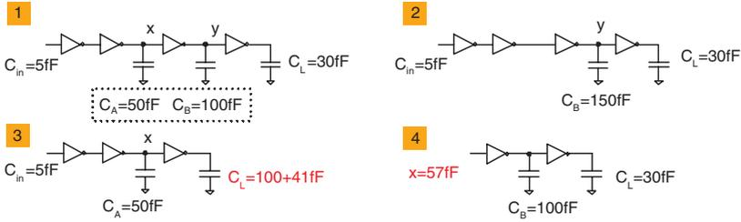
**Fig. 6.** Steps of the recursive procedure that handles multiple levels of interconnect
