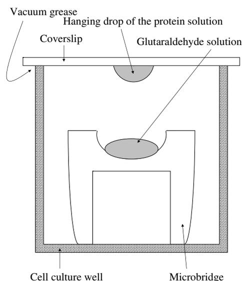
Fig. 2. Schematic diagram illustrating the entire experimental setup, used in the second protocol.
