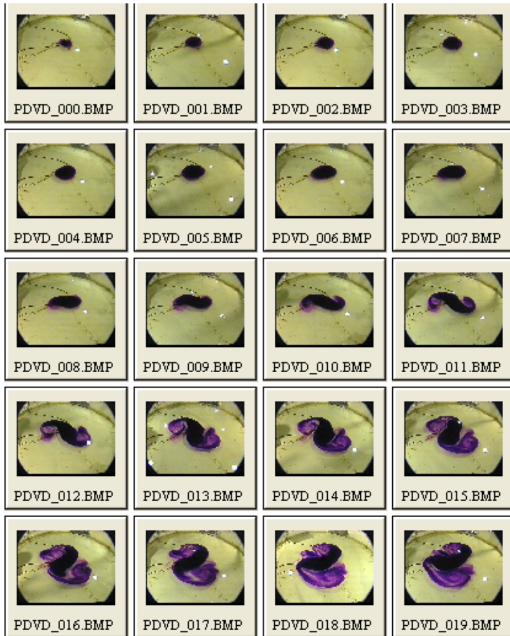
Figure 1. Successive photo of the evolution of the submerged gravity current. The rotation period is 60 s. The first photo was taken 30 s from the start of the buoyant plume flow. The time distance between each photo is half rotation period (30 sec). We observe that initially the spreading of the gravity current is axisymmetric, and that at about 3 revolutions the gravity current has the morphology of an ellipsoid. At about five revolutions, we observe the initial formation of two cyclonic vortices. At about six revolutions, the cyclonic vortices are well developed. At about 8 revolutions, the well-organized cyclonic vortex has moved away from the main gravity current and a process is under way for the production of two new cyclonic vortices.
