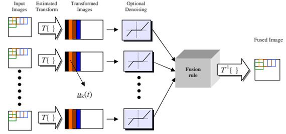
Figure 1. The proposed fusion system using ICA / Topographical ICA bases.
