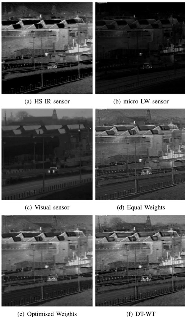
Figure 5. Optimal Contrast correction for the TNO Human Factors dataset. The optimal contrast selection scheme chooses to emphasize the contrast of the two Infrared images to the low-contrast night visual image.
