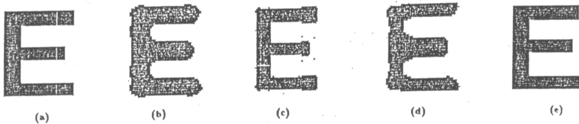
Fig.4 Noise-free reconstruction of a 60 \times 60 pixels letter E (a) Original image (b) Reconstruction with LM method on the whole image (moments up to 18 th order) (c) LM reconstruction with block segmentation (moments up to 18 th order ; subimage size 20 \times 20 ) (d) Reconstruction with ME method on the whole image (moments up to 6 th order) (e) ME reconstruction with block segmentation (moments up to 6 th order ; subimage size 20 \times 20 )
