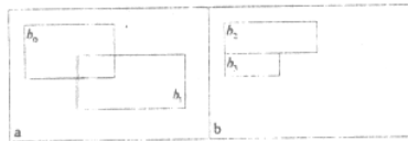
Fig. 2 (a). The relative positions of the blocks b_0 , b_1 according to a rectangular grid and (b). The execution of the function \text{COMAND}(b_0, b_1) , produces the blocks b_2 , b_3
