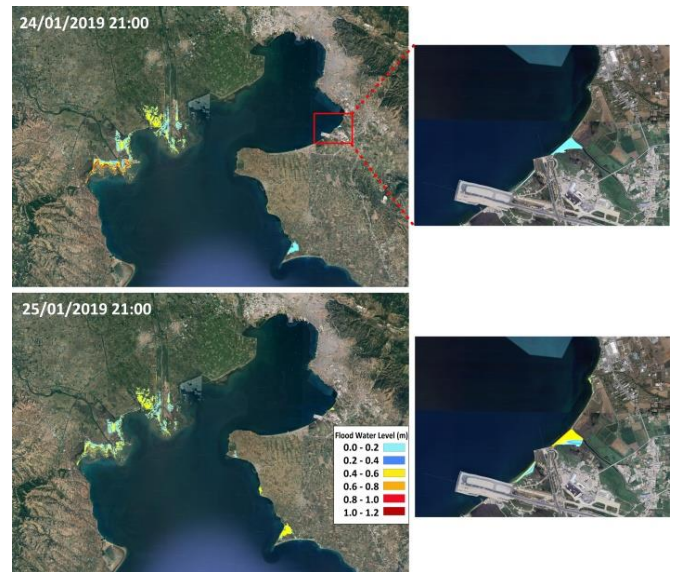
Figure 5. Forecast of flooded coastal areas and floodwater levels by CoastFLOOD model on 24-25/01/2019 (left). Zoom into the Macedonia Airport area (right).
