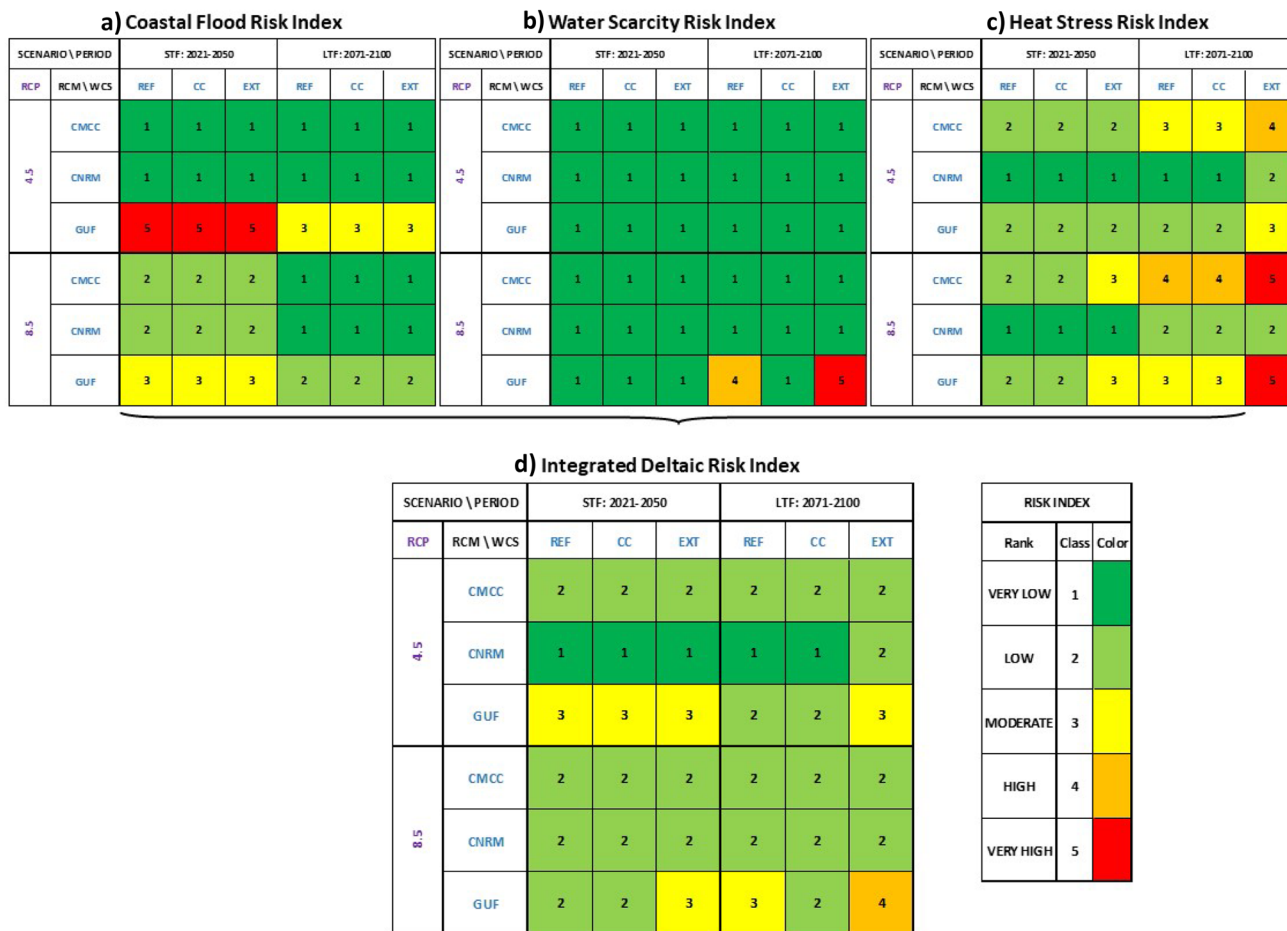
Fig. 12 Risk matrices for a CFRI, b WSRI, c HSRI, and d IDRI. Climate change impact identification is helped by graphing the differences in color scaling for each risk index, per: water consumption scenario (WCS: REF, CC, EXT), climate modeling input (RCM) for
