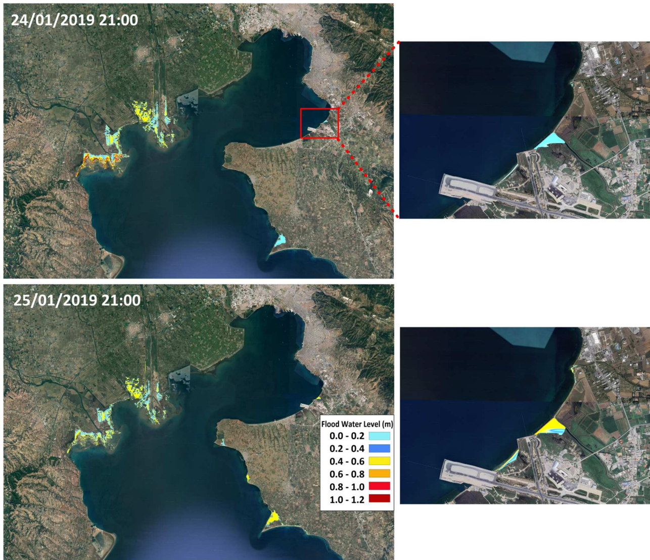
Figure 7. Inundated areas and Flood Water Level (m; above land elevation), derived from the coastal flooding forecasts (CoastFLOOD) on 24/01/2019 21:00 and 25/01/2019 21:00 (left panels). Details over Area 7 (Macedonia Airport) during the same dates are also shown (right panels).
