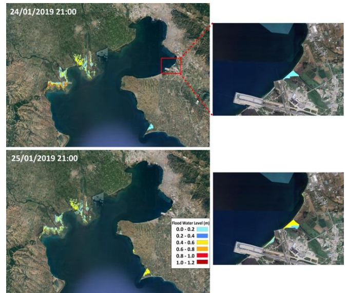
Figure 5. Forecast of flooded coastal areas and floodwater levels by CoastFLOOD model on 24/01/2019 and 25/01/2019 (left). Zoom into the Macedonia Airport area (right).
