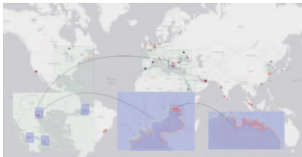
Fig. 1. Selected locations of 50 important ports around the globe and their corresponding data acquisition areas and bathymetries for each model (green for model H, purple for model A and densified near port area for model B).
