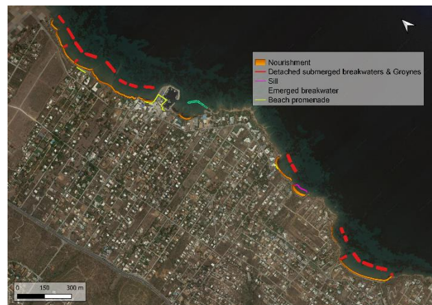
Figure 3. Layout of proposed coastal protection works.
