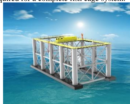
Figure 1. Rendering of the OS-Aqua cage system design
