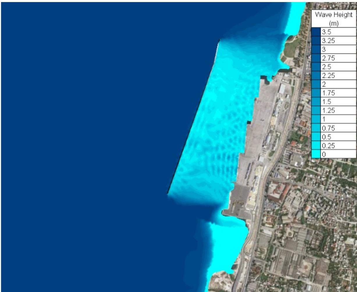
Figure 1. Spatial distribution of the significant wave height inside the New Port of Patra, Greece
